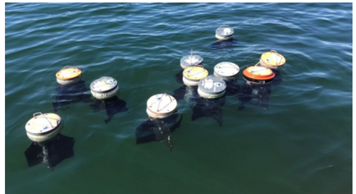
Figure 5: Surface drifters drift in the North Sea as a non-invasive tool for measuring currents, particles and water masses.
