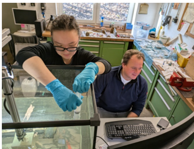
Figure 6: Maria Khon (L.; GEOMAR) and Ansgar Leefken (r.; URO) sampling a current flume experiment at the KR D S-H facility. The flume allows precise control and measurement of current speeds over a solid explosive fragment, and water samples are simultaneously collected over time to calculate dissolution rates.
